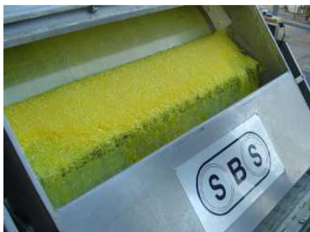
**Figure 2.** Sulfur pastilles at discharge.
