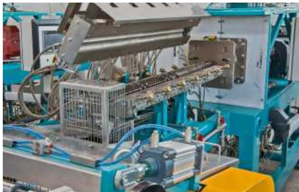
**Figure 1.** Mixing extruder for sulfur bio-fertilizer.
