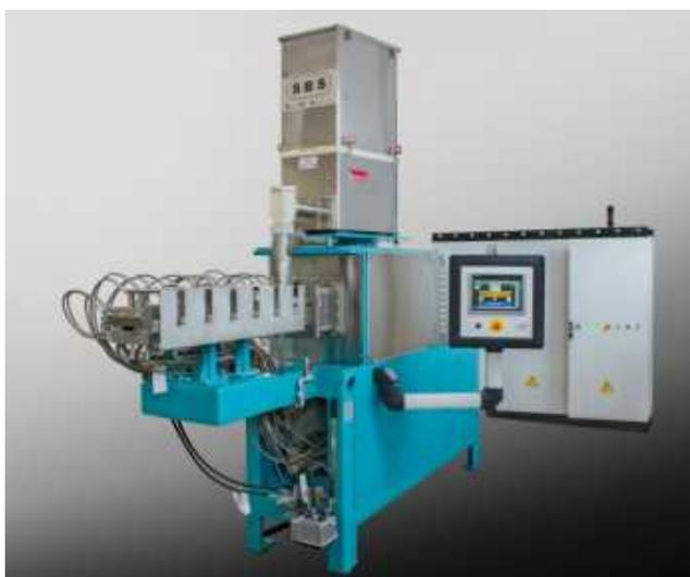
**Figure 6.** Industrial extruder closed.
